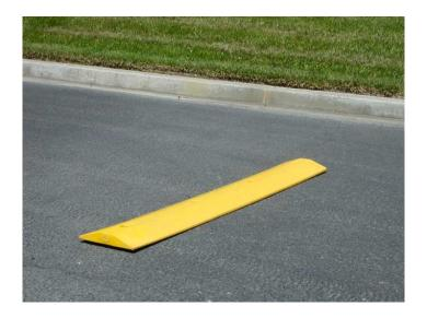
Designed to slow traffic in parking lots, driveways, construction sites and similar areas where high speeds can be dangerous. Bright yellow color improves visibility. Use for temporary or permanent installations. Concrete mounting hardware included (½" X 6" long concrete anchors). Asphalt installation kit available. Constructed of recycled polyethylene and polypropylene.
