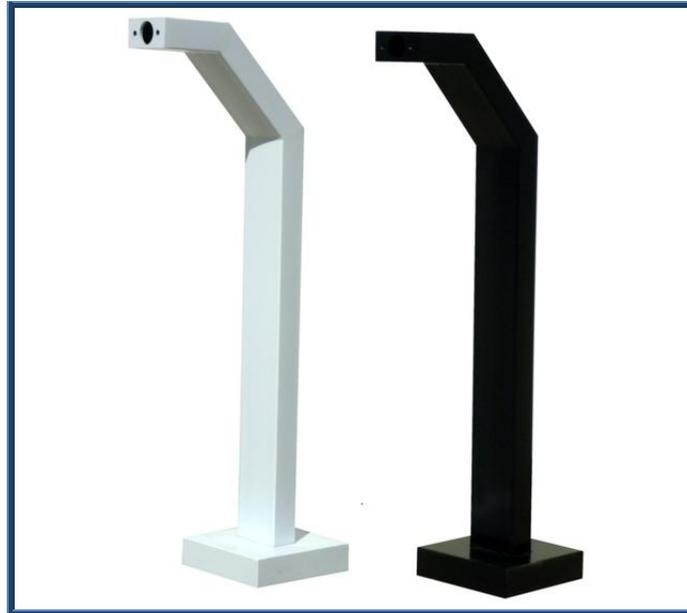
These pedestals are typically used to install card readers or intercoms at drive-up and pedestrian access points. Made of 2" X 4" rectangular steel tubing with an 8" X 8" base plate. A steel base plate cover is provided to conceal the mounting hardware. Housings and adapters are available for these pedestals to accommodate most access control devices such as card readers and intercoms.
