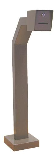
The model 307-1P magnetic card reader is a low cost, high quality access control device which is used primarily to control access to restricted areas where an electronic or computerized system is not needed. When the correct, durable coded plastic card is inserted into the card reader, a switch is activated. This switch can trigger automatic gates, electric door strikes and other access control devices.
