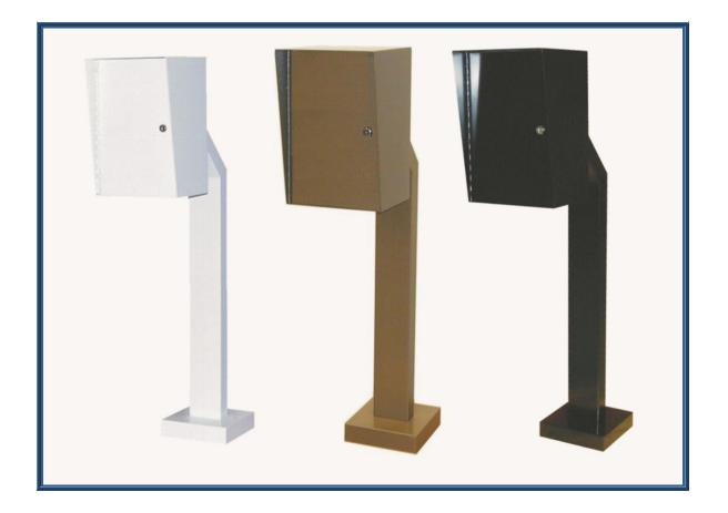
These housings and pedestals are used for the installation of card readers, intercoms and other devices at vehicular and pedestrian access points. Hinged door with cam lock provides both security and ease of access. Standard finish is either white, beige or black powder coat. Model 9050-1-1 includes Model 306-6, 36" tall pedestal and 9050-1BD, 14" H X 9" W housing.
