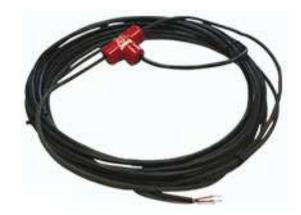
The PFL preformed vehicle detection loop is constructed of stranded wire conductors with XLP thermoplastic elastomer insulation jacketing. The outer shell is flexible nonmetallic 0.26" tubing. The vehicle detection loop includes electronic lightning protection. The lead-in wire is twisted, shielded and 50 ft. long.
