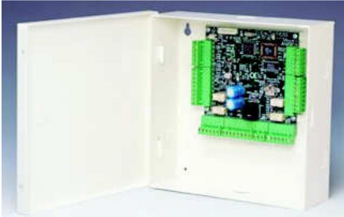
The SK-ACP-LE Advanced Control Panel is a highly sophisticated, yet simple to use, two door access control unit. The unit accepts readers that have a Wiegand output with almost any card technology, including Proximity, Touch Card, Wiegand, Magnetic Stripe, Bar Code, Optical, and Biometric. Each of the two doors controlled by the unit is completely independent of the other and is configured, programmed and viewed separately. Each has a separate node address.
